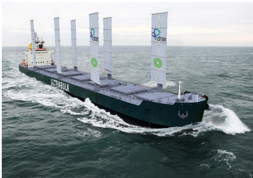
Picture 02. Panamax size Wing Sail retrofit bulk ship may be sailing soon. /Photo credit/permited by: Smart Green Shipping Alliance, Diane Gilpin, 22.3.2019
