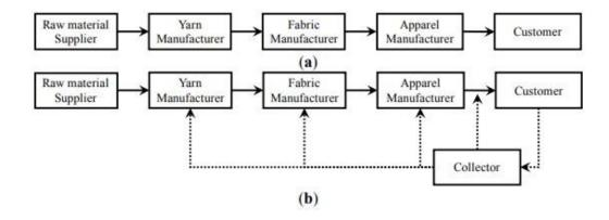
Figure 6: The difference between forward and closed-loop supply chain (Jisoo Oh, Bongju Jeong, 2014, 24).
