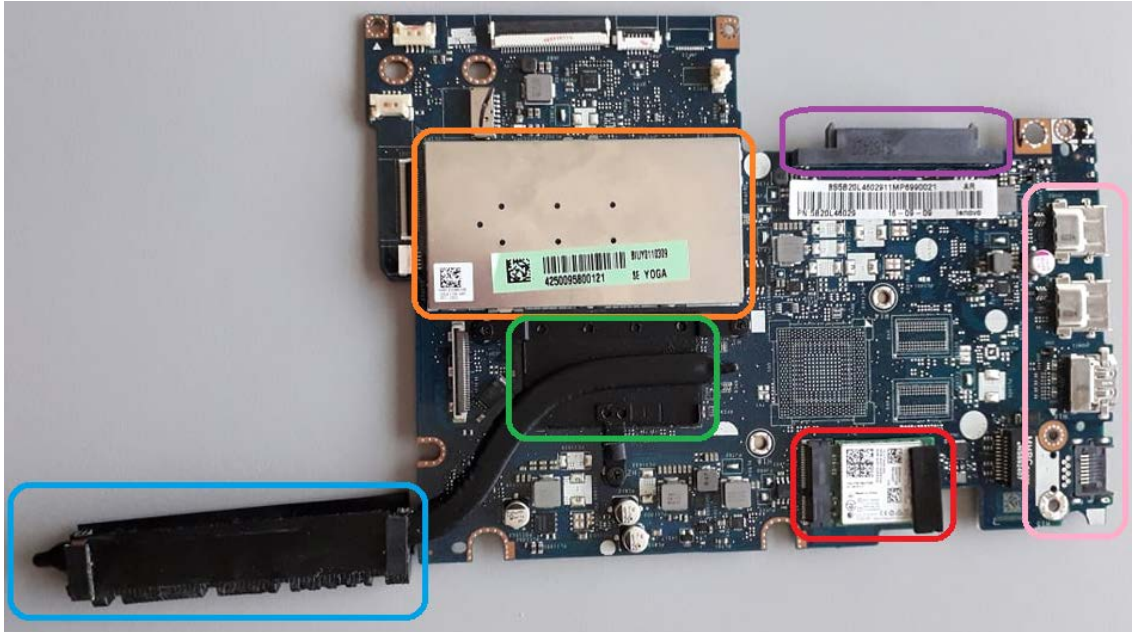
Figure 21: Motherboard with components: heat sink (blue), GPU cooling plate (green), RAM (orange), LAN card (red), I/O plate (pink), SATA 7+15 pin connector for the SDD disk (violet)
