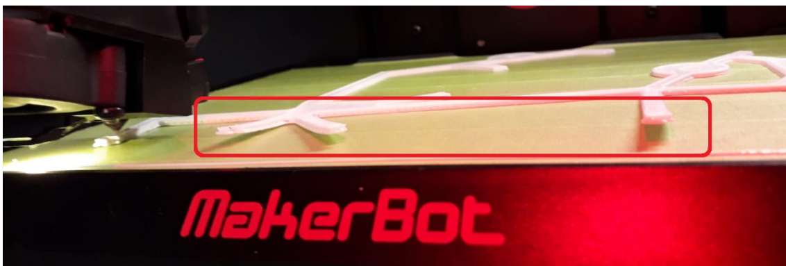
Figure 45: Wrapping of the Part SDD of the supporting structure (highlighted in red)
