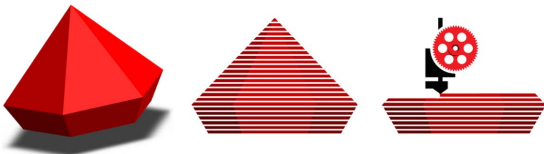
Figure 1: A 3D model presented as a set of slices (Shropshire 3D Printers)
