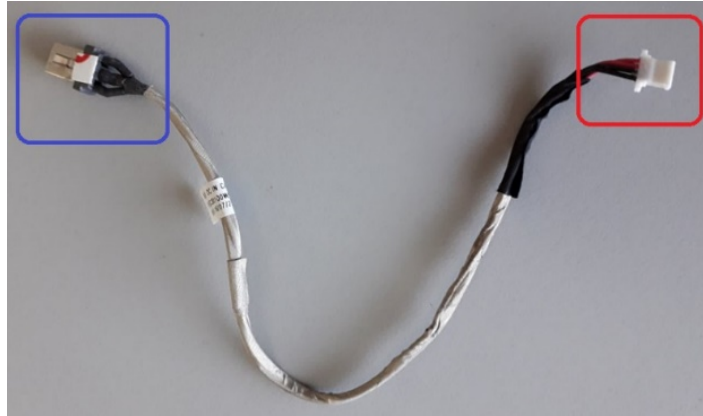
Figure 26: Power cord plug: connector for the charger (blue), connector for the motherboard (red)
