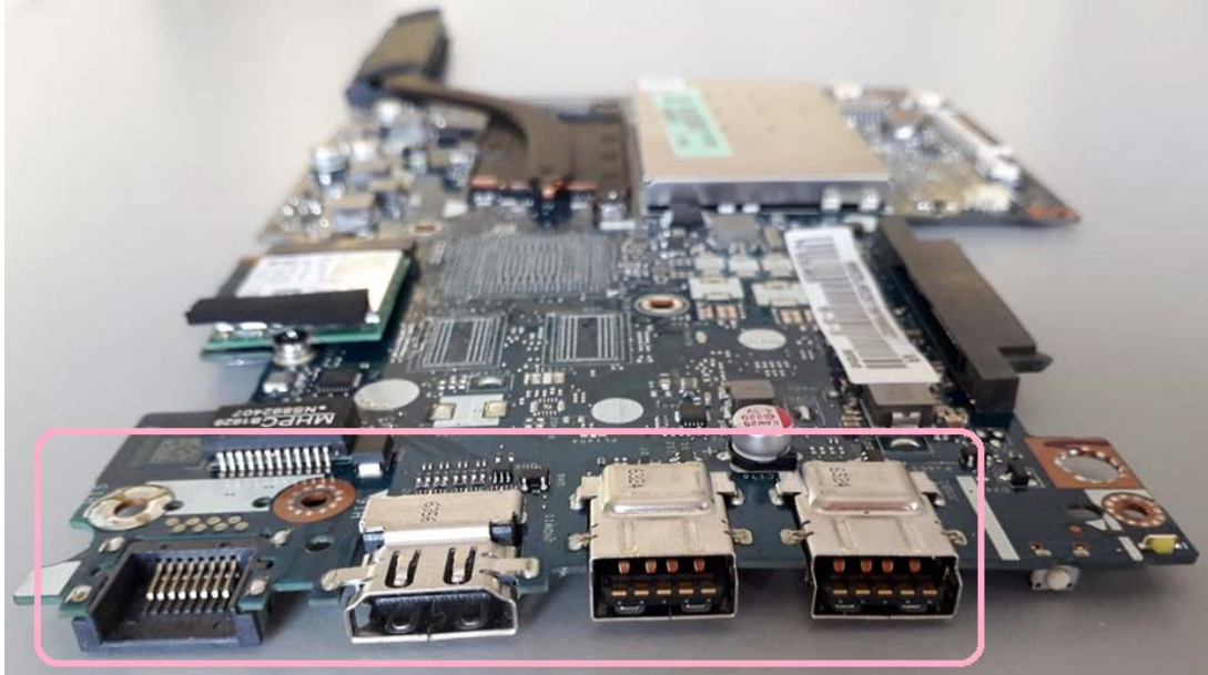
Figure 23: I/O plate on the motherboard, from left: internet connector, HDMI, and 2 USBs
