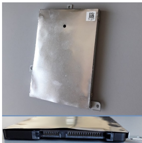
Figure 22: SDD Disk (top), and SATA 7+15 pin connector (bottom)
