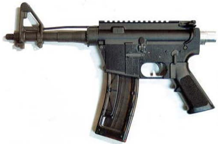
Figure 5: A 0,22 caliber gun, partly manufactured with 3D printed plastics (Lipson & Kurman 2013 p. 128)
