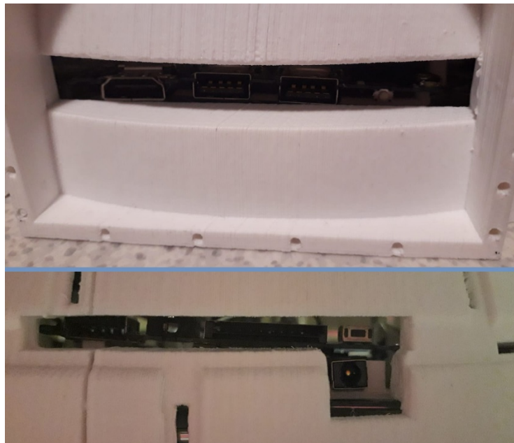
Figure 54: Positioning of the I/O plate (top) and I/O module (bottom) in the cut outs of the igloo casing
