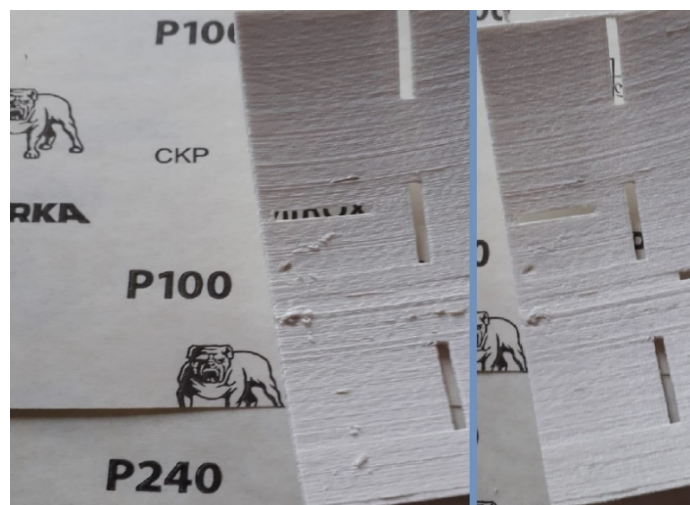
Figure 47: An example of improvement of the surface quality: before sanding (left), after sanding (right)
