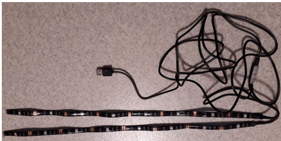
Figure 31: Two stripes of LEDs and their power USB connector
