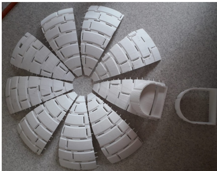
Figure 43: All 10 parts of the igloo casing
