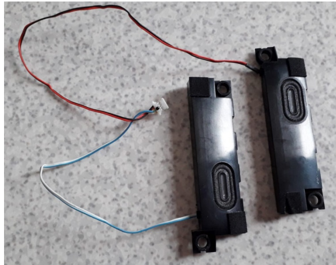
Figure 30: Speakers and their shared connector
