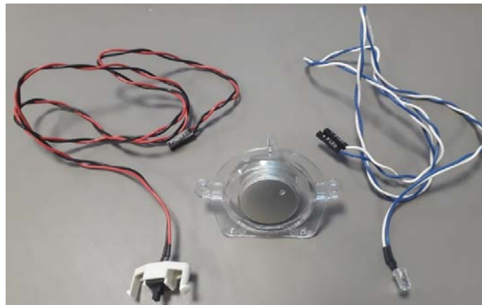
Figure 27: The parts of the power button: switch (left), plastic button (middle), and LED (right)
