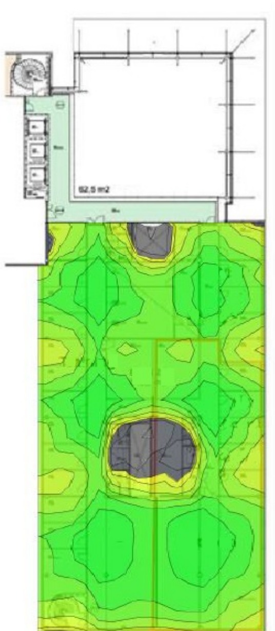
Figure 16 Predicted 5 GHz coverage in Helsinki site Area 1 and Area 3 (Wi-Fi Network report Helsinki 2019)
