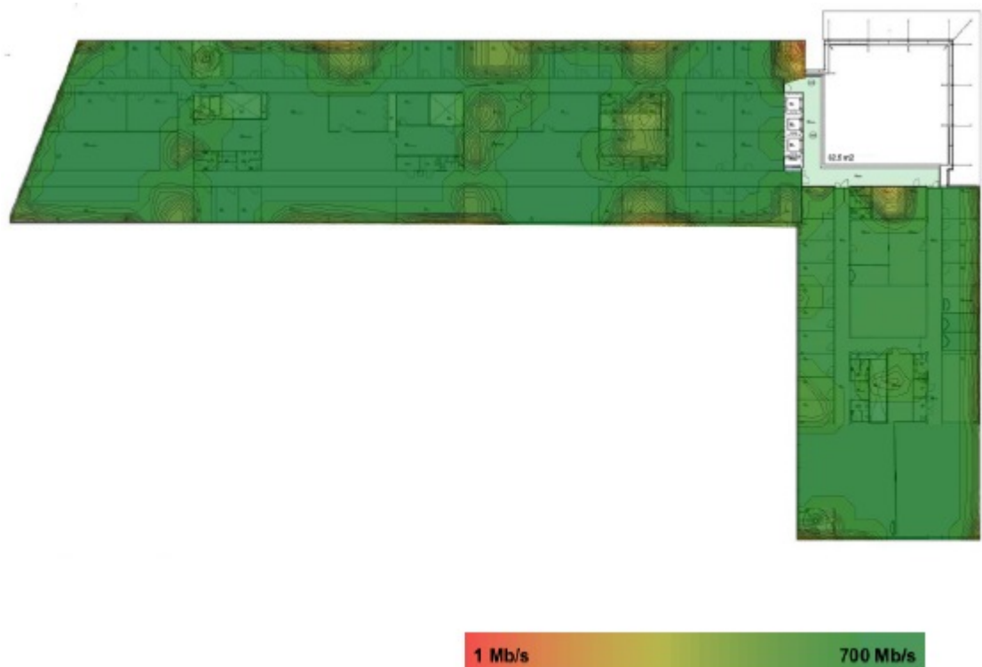
Figure 26 Data Transfer Rate for 5GHz in Helsinki site Area 2 and Area 4 (Wi-Fi Network report Helsinki 2019)
