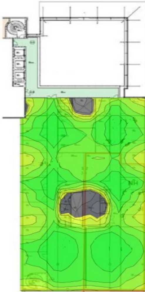
Figure 4 predicted coverage on Helsinki Area 1 and Area 3 (Wi-Fi Network report Helsinki 2019)
