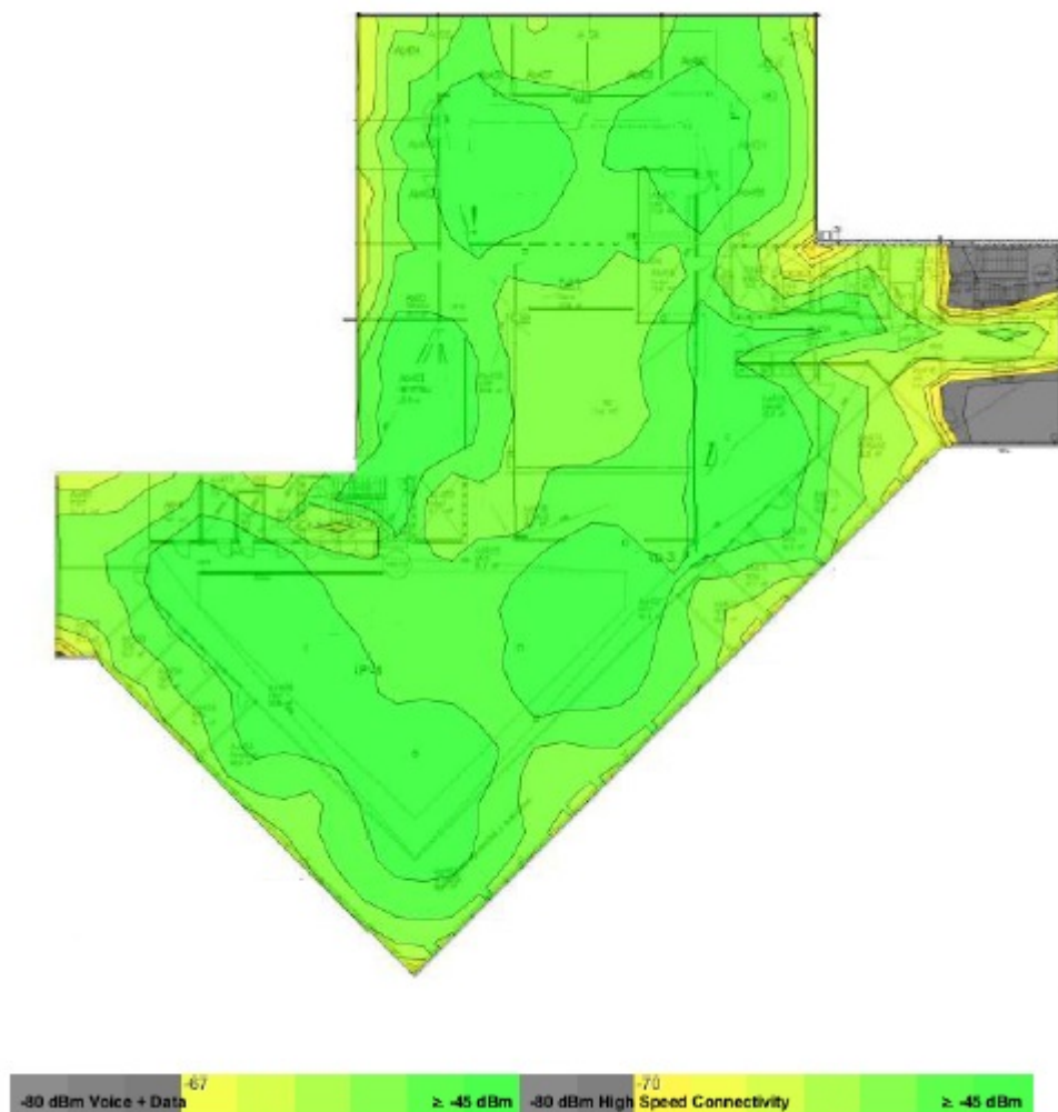
Figure 28 Signal strength in Jyväskylä site for Area 1 and Area 2 (Wi-Fi network report Jyväskylä 2019)
