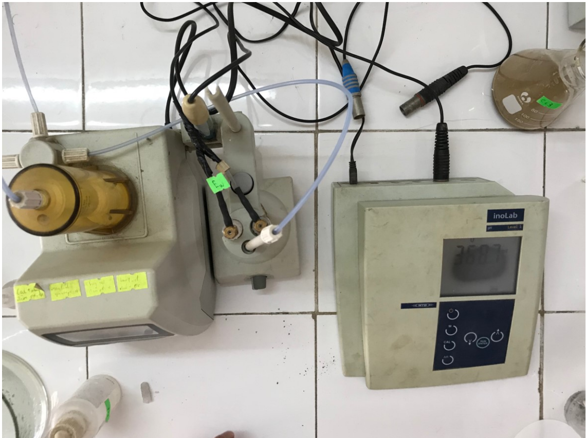
FIGURE 6. inoLab pH Level 1 and redox potential sensors
