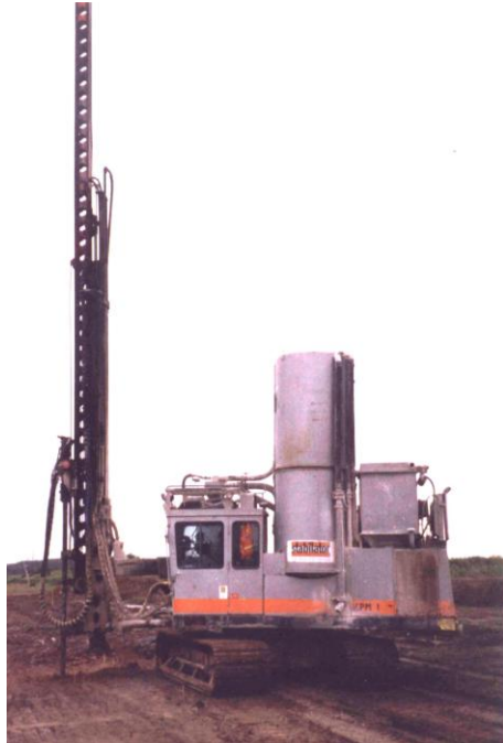
Figure 3.4.1a Deep dry mixing plant with on-board binder silos, air drier and compressor
