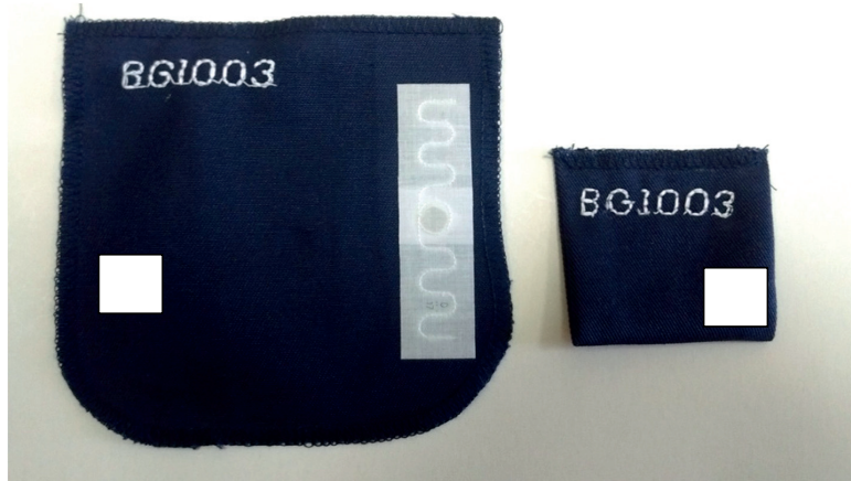
Figure 3.3. Fabric sample a) with ironed RFID tags, b) with sewn RFID tags.
