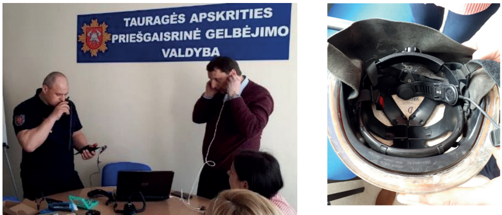
Figure 7.16. The moment of testing and helmet with integrated earpiece – bone microphone
