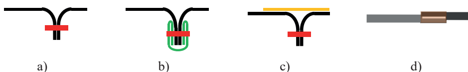
Figure 7.3. Seam types in CPC suits: a) stitched seam; b) bound seam; c) stitched and taped seam; d) welded seam [128]
