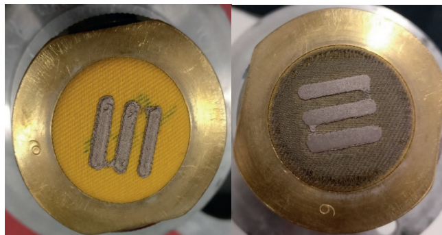
Figure 6.12. Initial specimen and after breakdown specimen (after 13000 rubs) of cooper PLA sample on fabric F1
