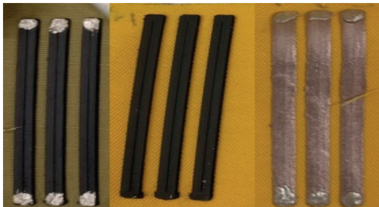
Figure 6.16. Washed 2 times Graphene PLA on fabric F1, F2 at 75 °C
