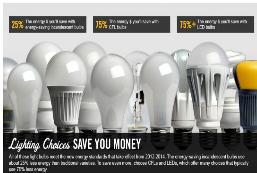
Figure 15. Comparison between halogen, CF, and LED light bulbs and the amount of energy they save (Lighting Choices to Save You Money, n.d.)
