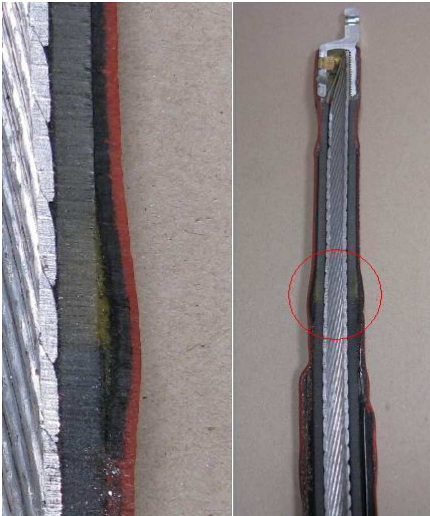
Figure 19. Cutting point of the cable screening
