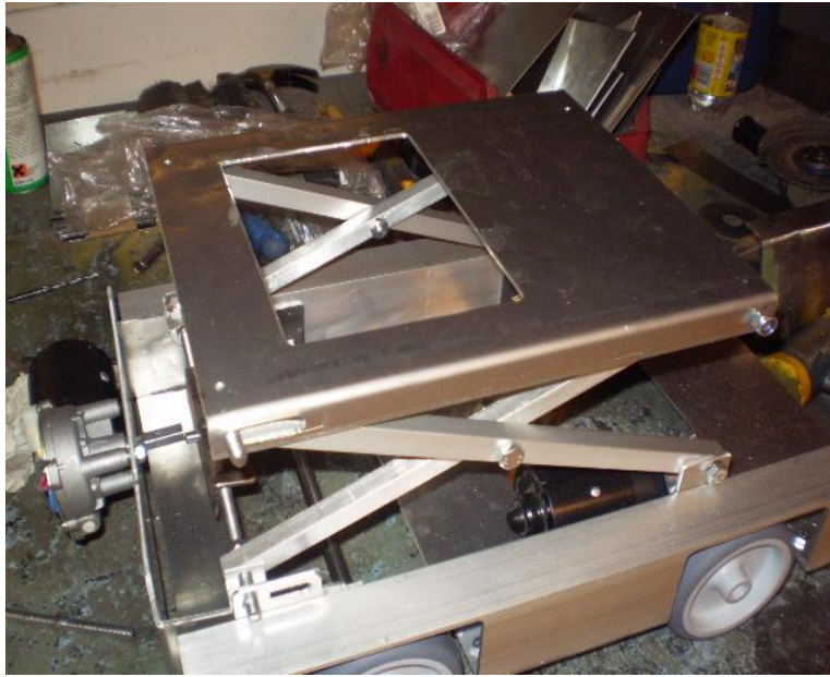
FIGURE 66 Lifting system on the vehicle version 1
