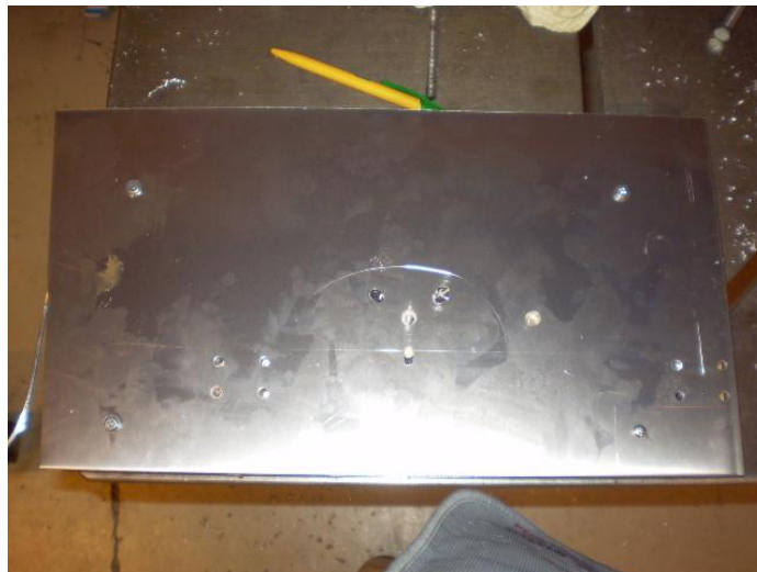
FIGURE 77 Sheet metal piece fixed to the wood plate. Holes have been already milled.
