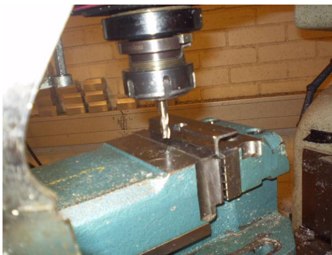
FIGURE 71 Milling cavities into the steel profile.
