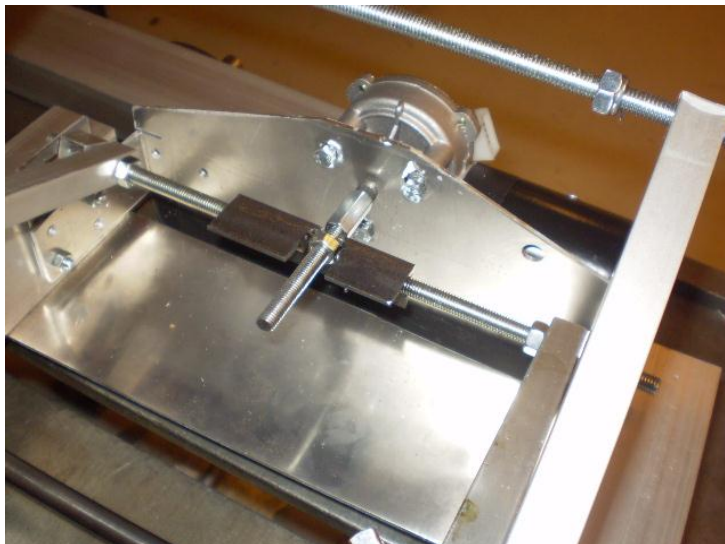
FIGURE 83 Assembled lifting system motor on vehicle version 2
