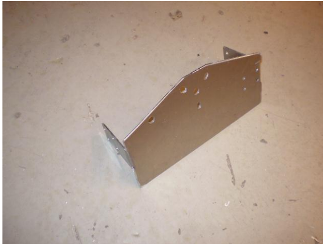
FIGURE 79 The ready lifter motor support piece
