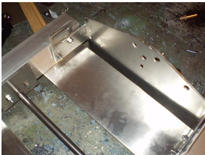
FIGURE 81 Fixing the motor support
