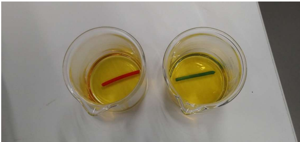
Figure 23. Setup of the test. The specimens of polymers have been submerged in the oil
