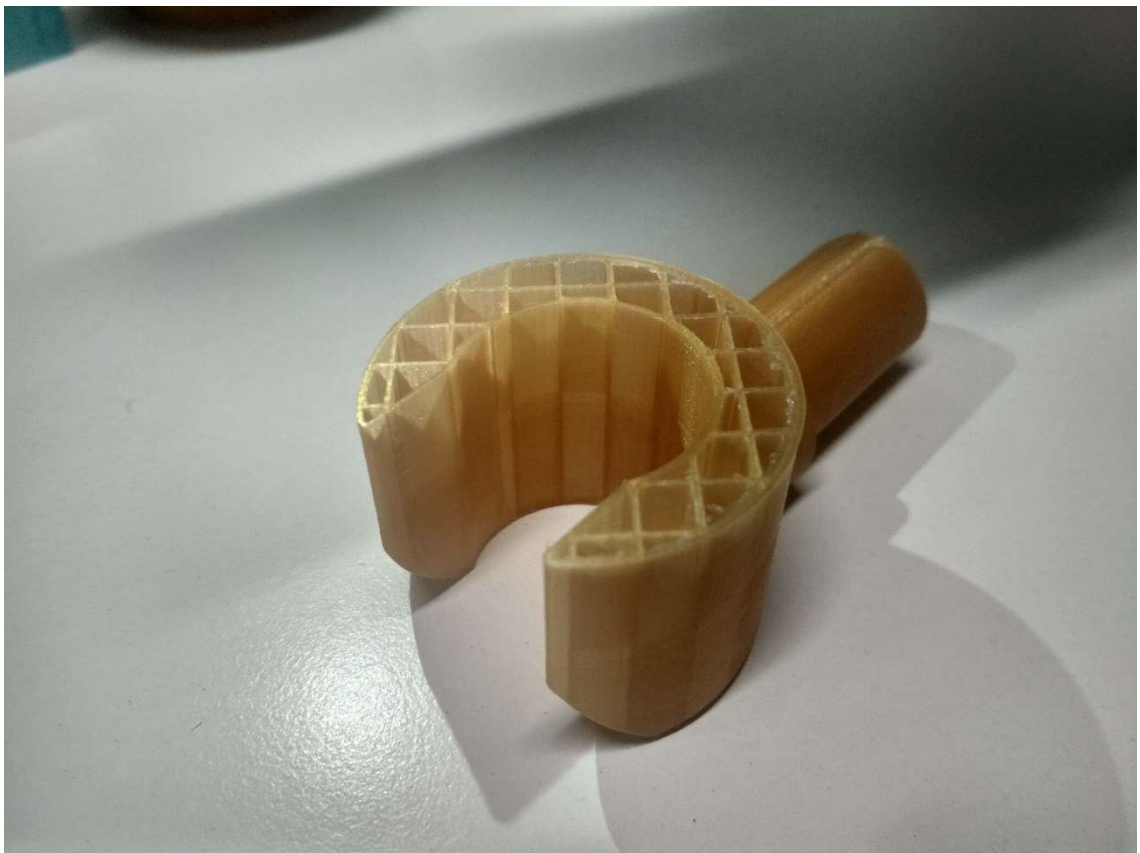
Figure 4. A printer LEGO hand with visible internal rectangular structure (Dobryakov 2019)
