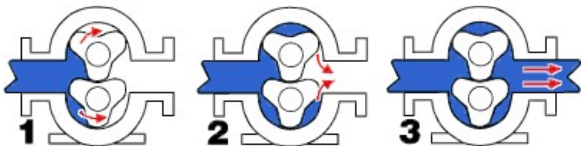
Figure 7. Scheme of a generic rotary lobe pump: 1. the liquid is flowing into the cavities that are created by the rotating lobes, 2. the liquid is moving in the cavities between the lobes and the casing of the pump to the outlet side of the pump, 3. the liquid is continuously flowing through the outlet port (Pump School 2017)
