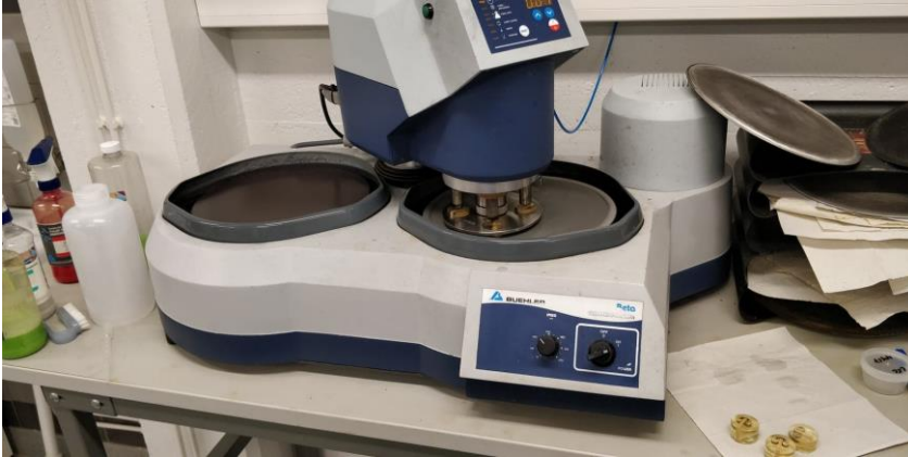
FIGURE 14. Instruments used for polishing the surface of microscopic test samples
