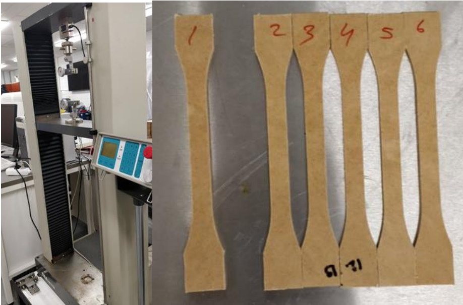
FIGURE 13. Universal tensile testing machine & Sample specimens for tensile test
