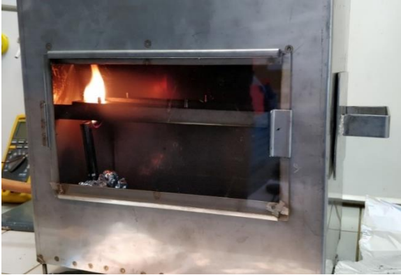
FIGURE 16. Horizontal burning test of wood plastic composites
