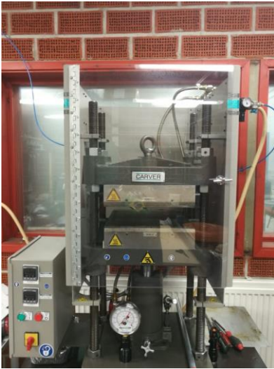
FIGURE 12. Manual hydraulic laboratory hot press used to produce composite plates
