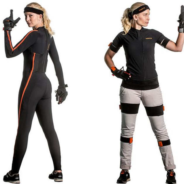
Picture 4. Performer wearing full-body (left) and strap-based (right) inertial mocap suits (Xsens, 2019c).
