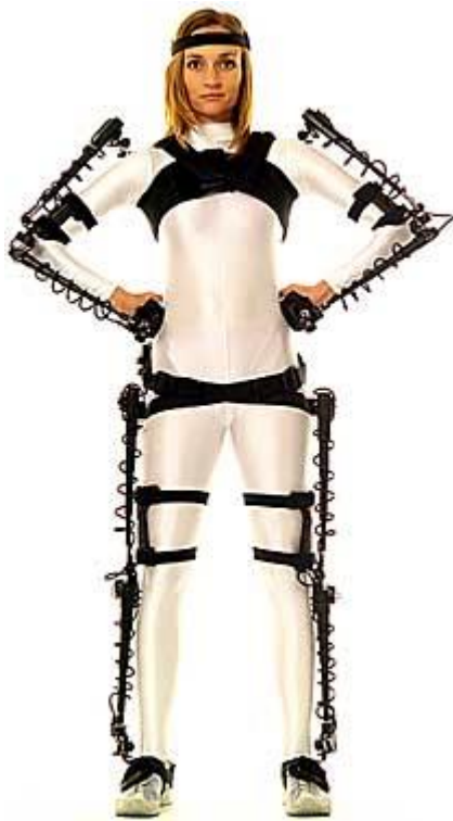
Picture 2. An actor wearing a mechanical mocap suit (Metamotion, 2019c).
