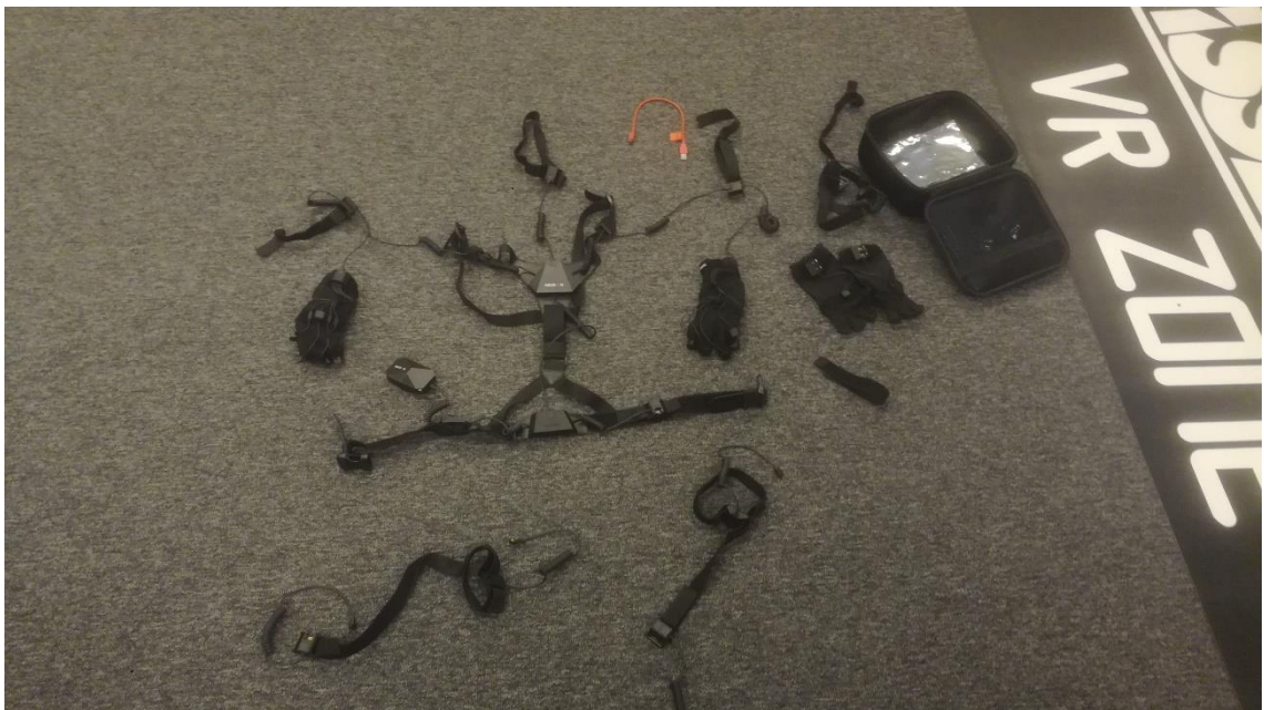
Picture 7. Perception Neuron mocap suit unboxed with all the components layed on the floor.
