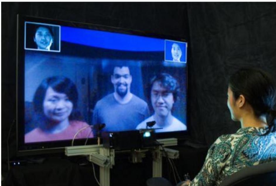
Figure 2. Real-time 3D scanning system using 120Hz video projector and camera (Lång 2009)
