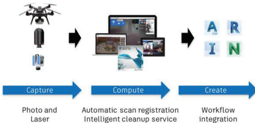
Figure 7: The steps to acquire information and implementation with BIM technology in as-built projects and modeling heritage, (Adapted by Author)
