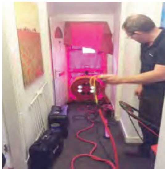
Figure 11: Pressurisation test (Morgan, 2018)
