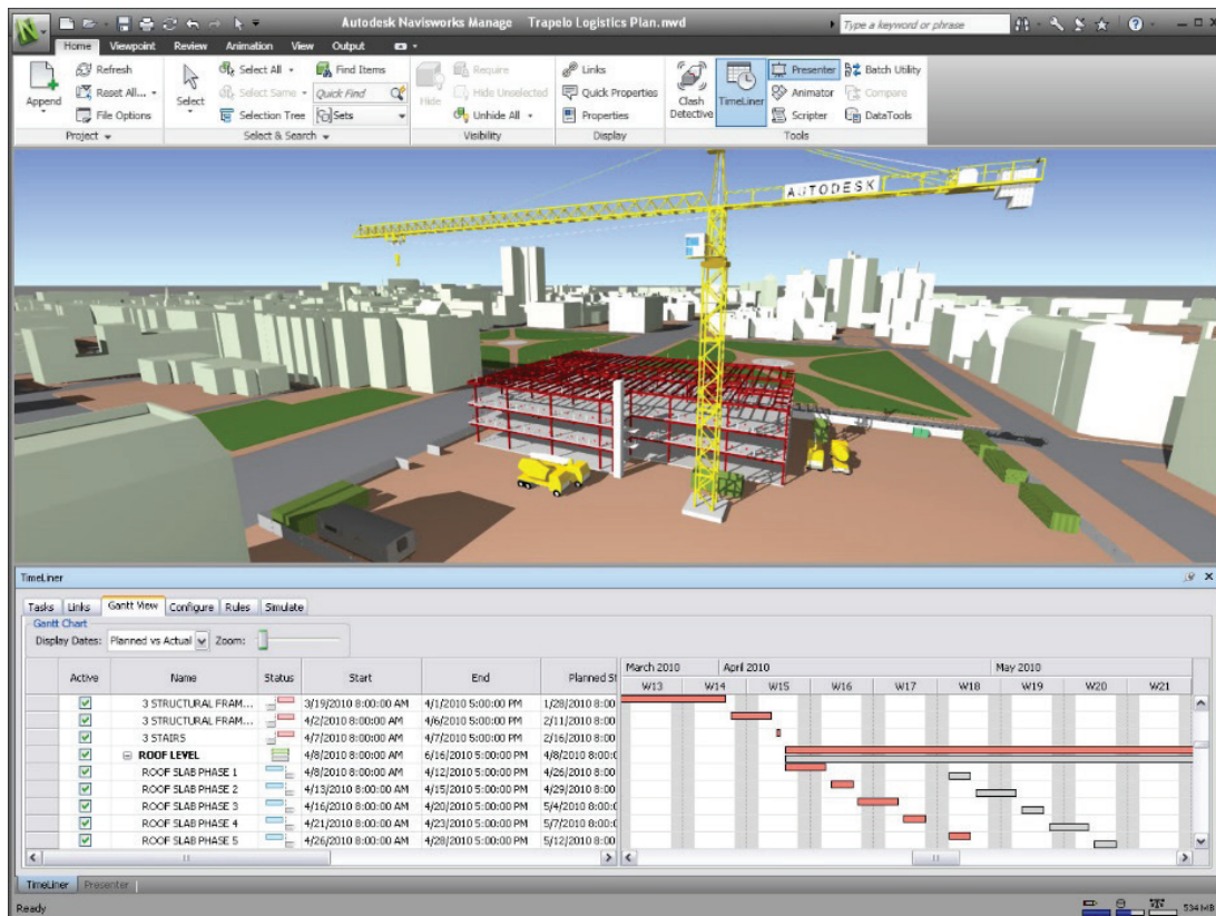
Figure 8 : Integration of BIM models, project management models and production of 4D model (Autodesk, 2019)
