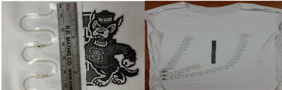
13.att.Conductive LED and ECG interconnect circuits laminated on shirt [50]
