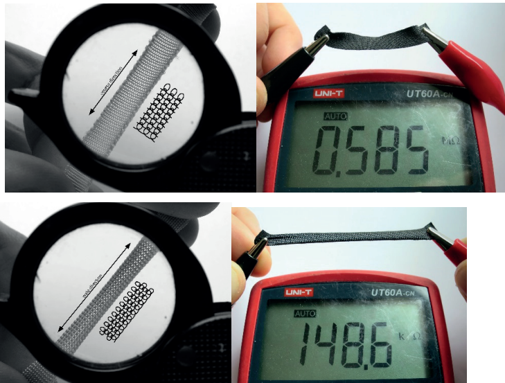
7.fig. Electro-stimulation of knitted structure [28]
