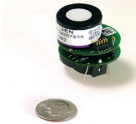
37.fig. Texas Instruments gas Sensor Platform with bluetooth Low Energy Evaluation Module [111]
