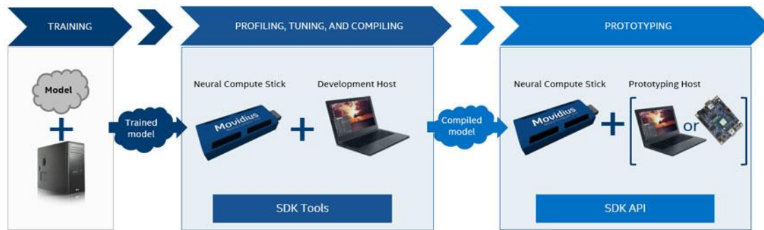
Figure 17. The development workflow diagram for the Intel's Neural Compute Stick [32]
