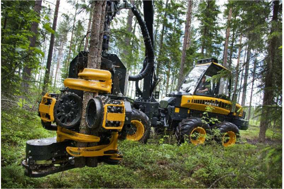
PHOTO 14. Ponsse H6 harvester head is optimal solution for multi-stemming small trees. (Ponsse)
