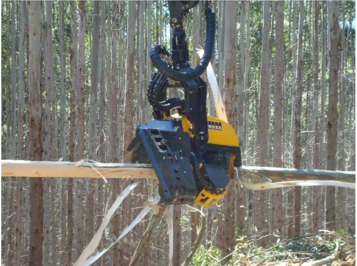
PHOTO 11. Ponsse H7euca harvester head. (Ponsse)
