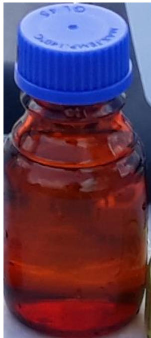
PICTURE 2. 250ml - grab bottle for sampling in the KgM-project (Eglinski 2019)
