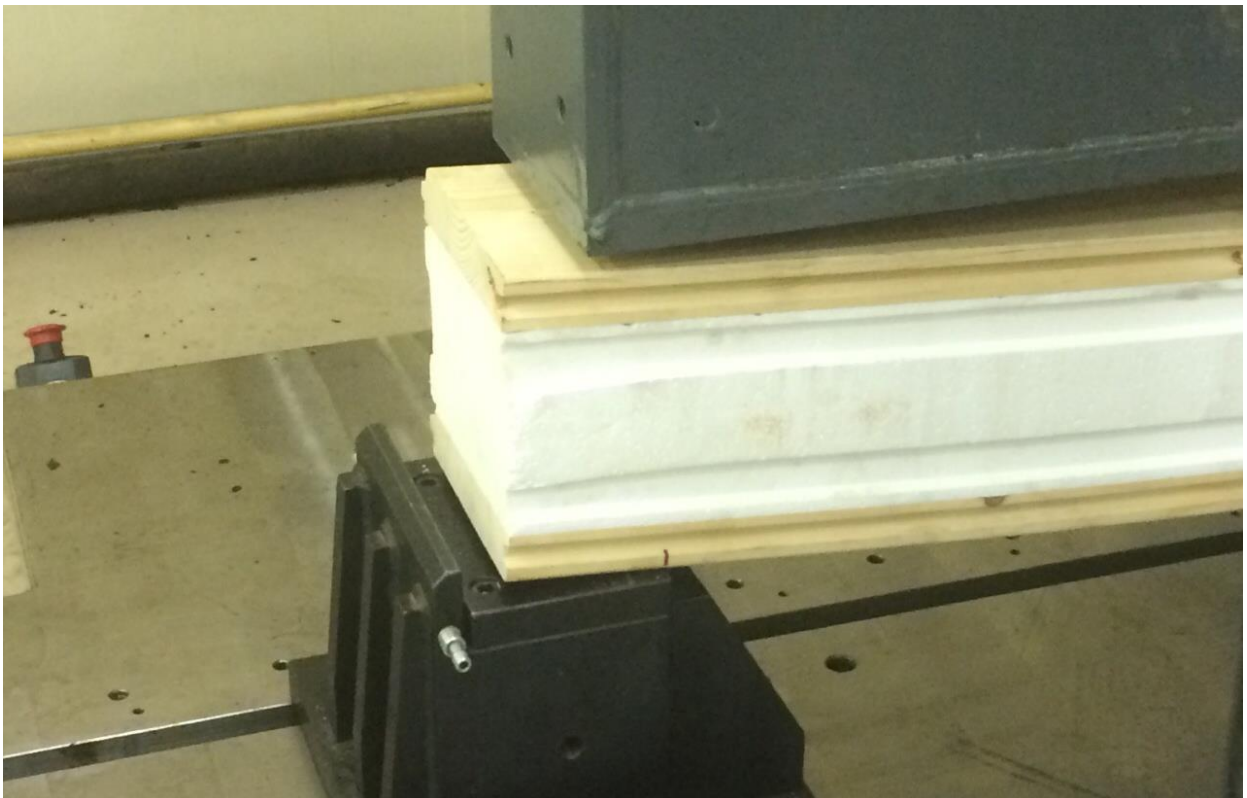
Figure 67. Beam on the support after loading
