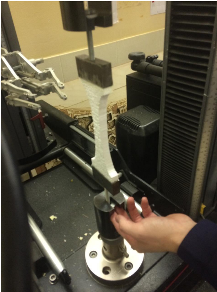
Figure 53. Determination of tensile strength of the polystyrene
