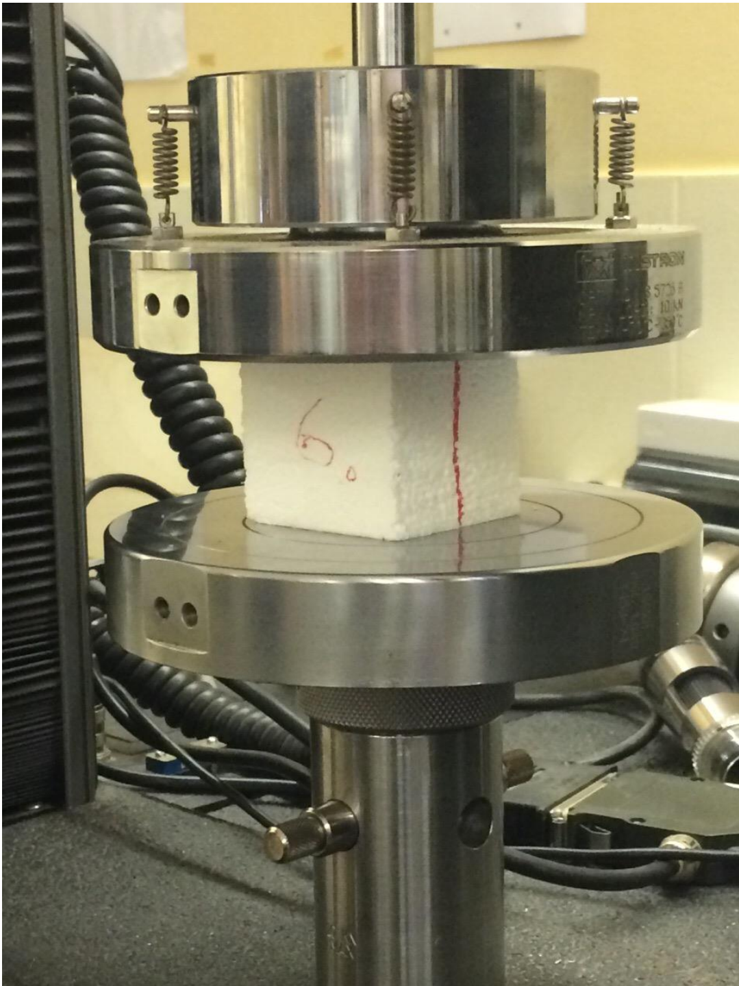
Figure 55. Determination of modulus of elasticity
