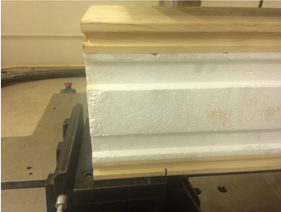
Figure 59. Beam on the support 100 mm
