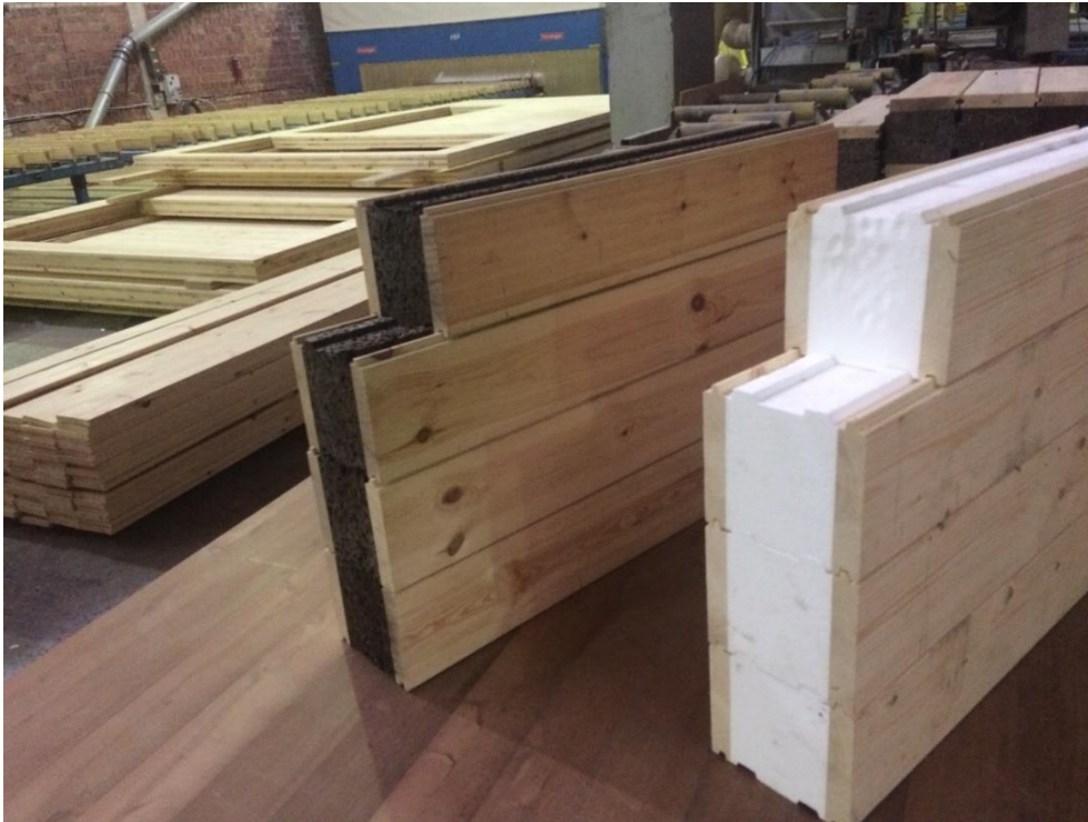
Figure 10. Two versions of beams with insulation from cork and polystyrene
