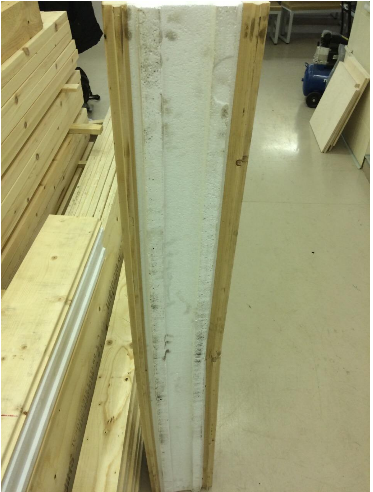
Figure 65. Beam after destruction in the compression zone
