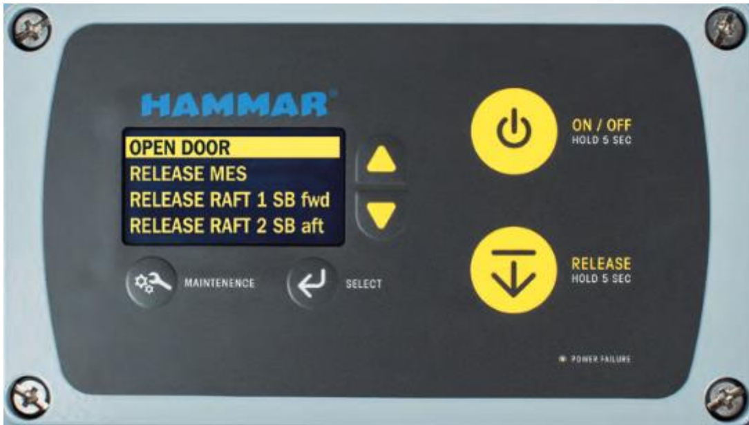
Figure 12 Hammar liferaft remote release panel. Photo CM Hammar
