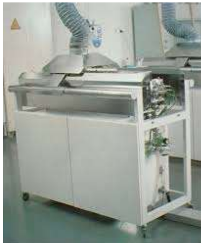
Figure 4 The first commercial ALD reactor model F-120 (Suntola's private collection.)
