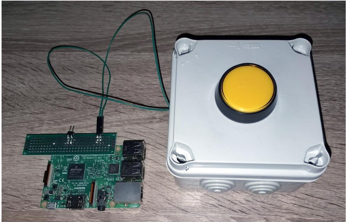
Figure 13. Raspberry Pi 3B with connector card and a button box
