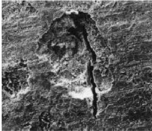
Fig. 3: Pitting induced stress corrosion cracking
