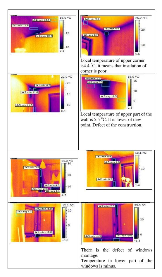
Figure 1. Thermograph of internal surfaces of premises.
