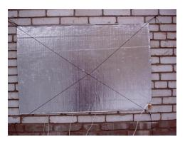
Figure 5. Flat heater, which provides stable thermal regimes.
