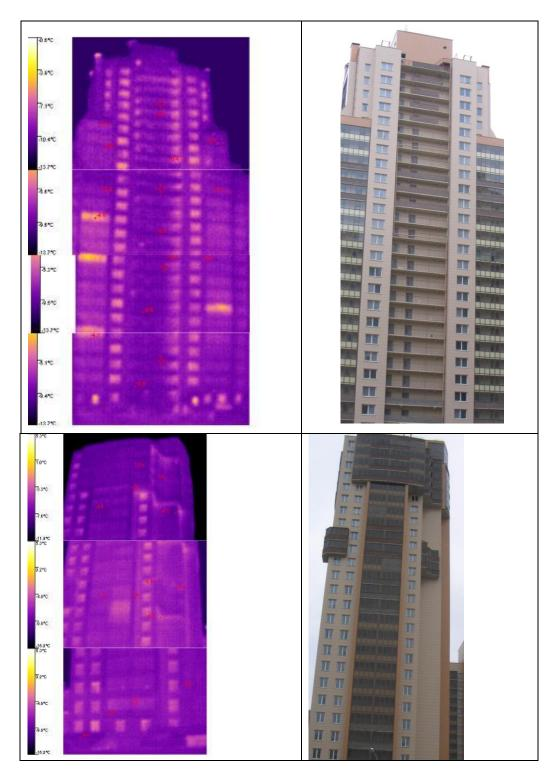
Figure 2. Thermograph of external surfaces of premises.
