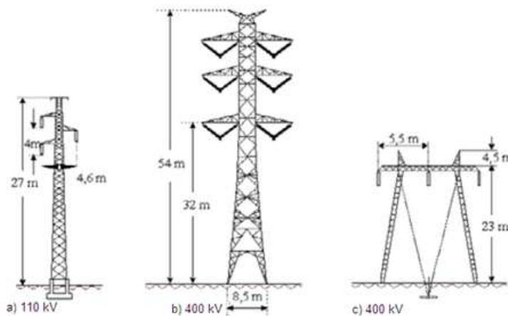
**Figure 4. Steel tower structures**
