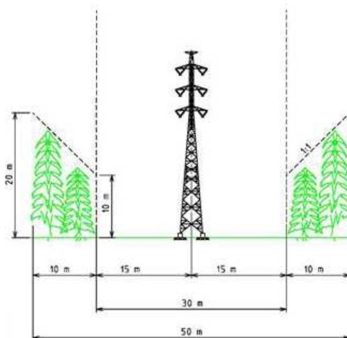
**Figure 7. Right of way for self-supporting tower**
