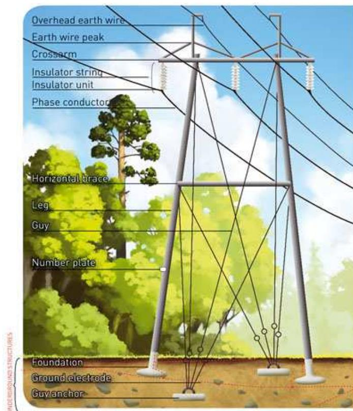
**Figure 5. Main parts of the guyed portal tower**
