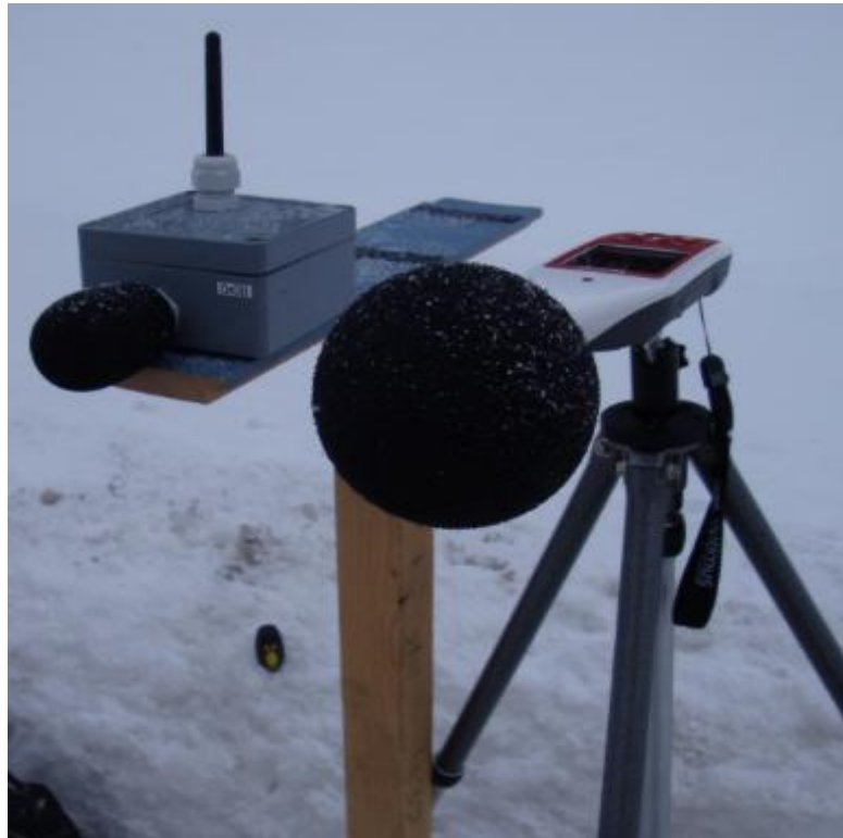
Figure 5: Our designed node work with standard calibrator
