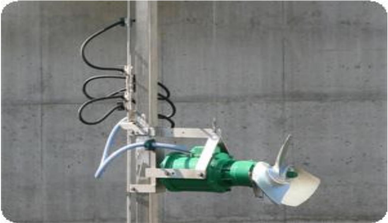
Figure7. Submercible agitator [14]
