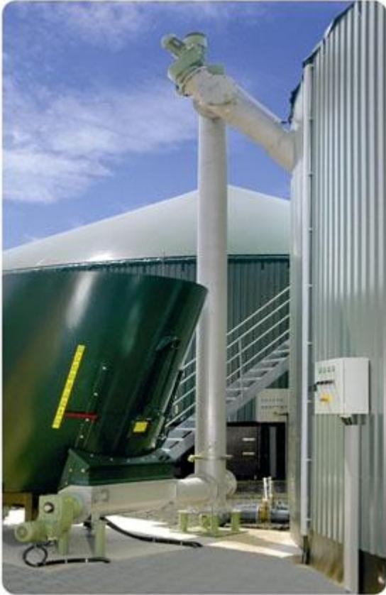
Figure5 .Screw loader and dozer of biomass [12]
