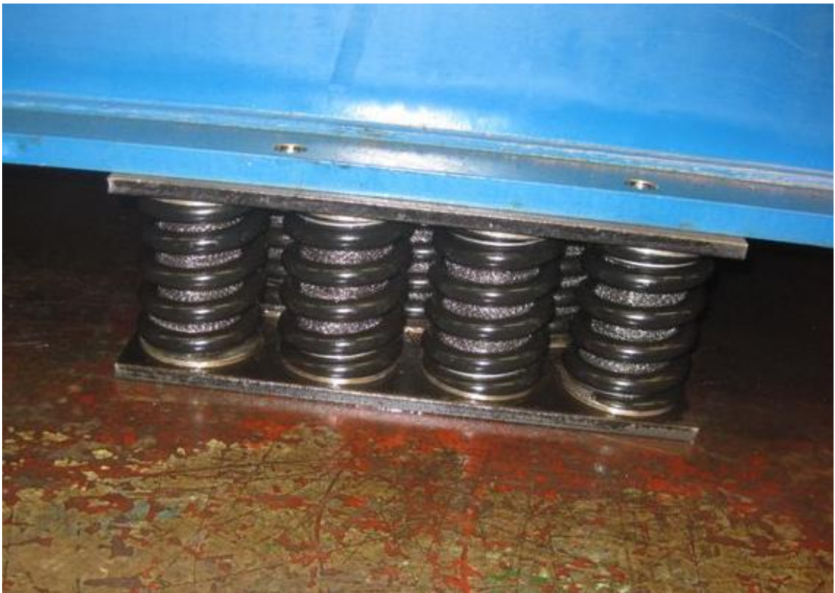
Figure 3. Spring mounting used by Wärtsilä in the test run.
