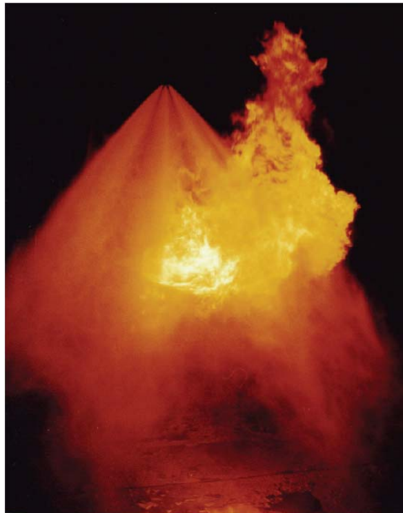
Figure 3. Picture from HI-FOG® fire test (from HI-FOG® sales brochure)
