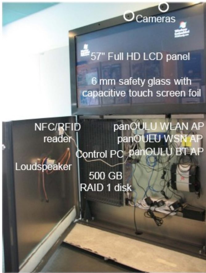
FIGURE 14. Structure of indoor UBI-hotspot (11, p. 2)
