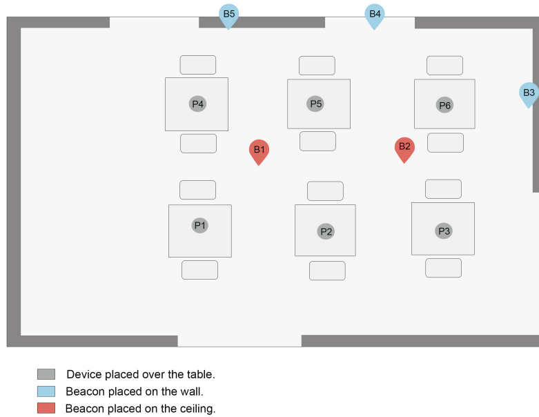
Figure 14. Space set up for the fourth test, Beacon placement and reading positions.
