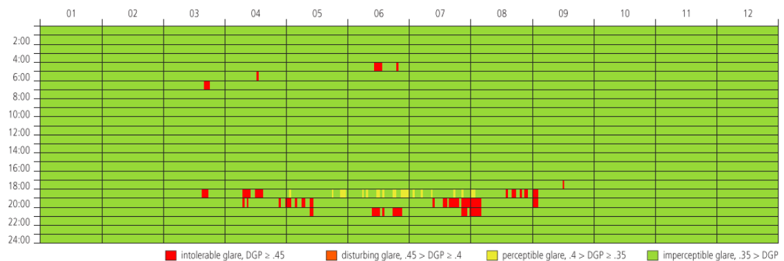
Figure 27. DGP values simulated by DIVA for the modified design.
