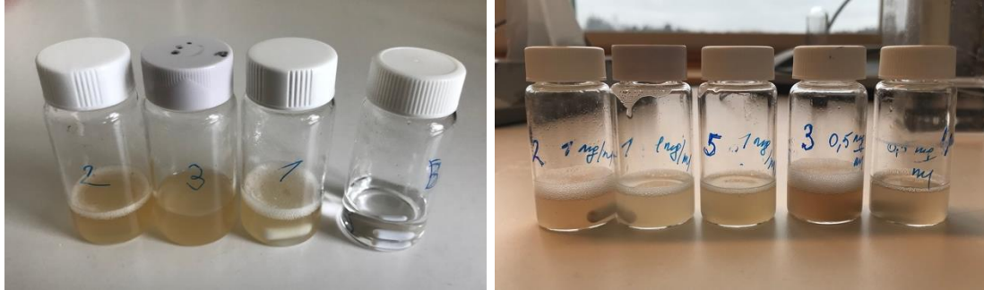
Figure 2: Samples with 1 mg/ml (right), 0.5 mg/ml (left) and 0.1 mg/ml (left) of Creon concentration after digestion in incubator for 24 hours
