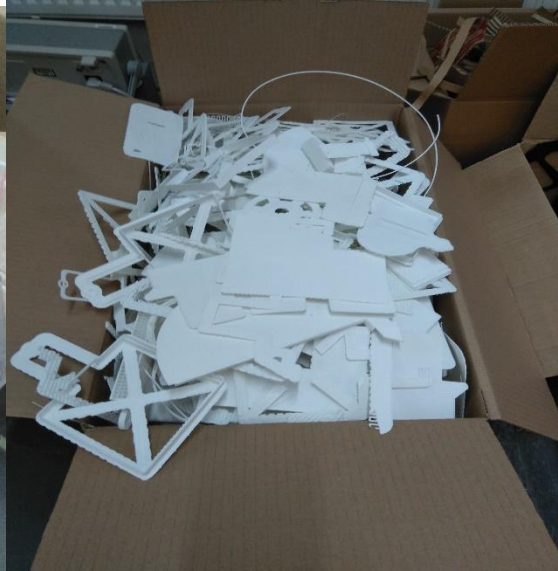
Figure 12 3D printed failed parts(white)
