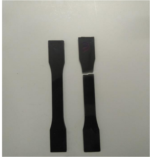
Figure 23 Black sample after tensile testing
