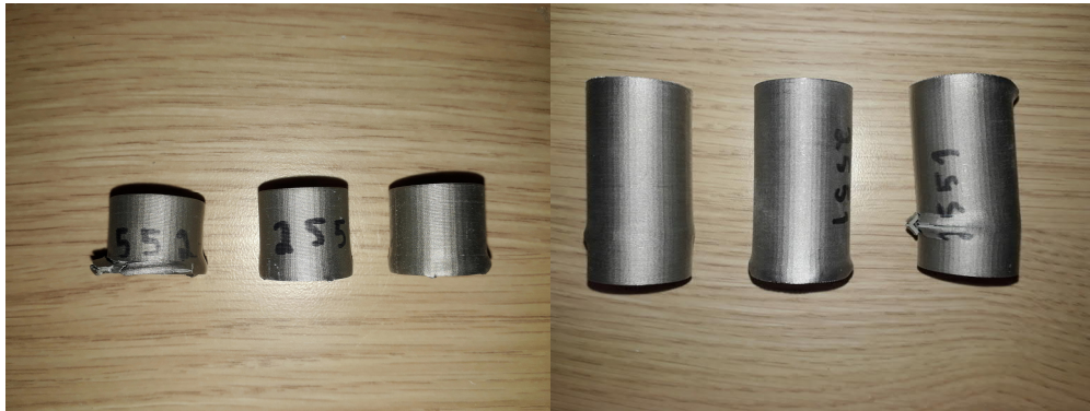
Figure 54. Compression test samples after the test, CS1 on the left and CS2 on the right.
