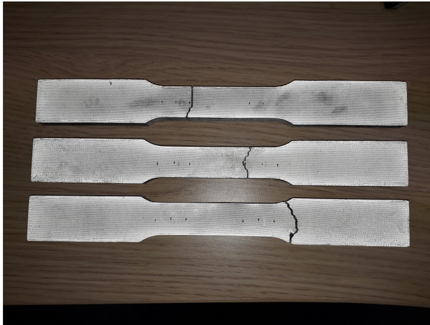
Figure 41. Test sample series TS11, where can be seen that one sample is broken outside the measurement zone, although the strength to break the sample did not deviate from others.
