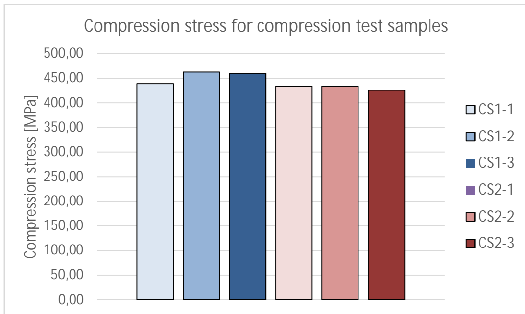
Figure 56. Compression stress chart for compression test samples in series CS1 and CS2.
