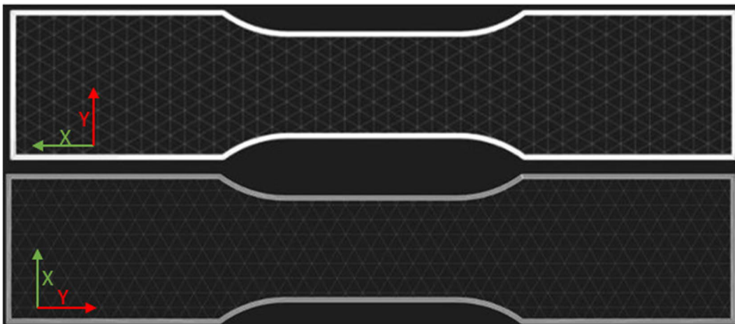
Figure 60. Cross-section views from Eiger, TS1-X on the top and TS1-1 on the bottom. This demonstrates that the infill structure has a huge impact to the strength.
