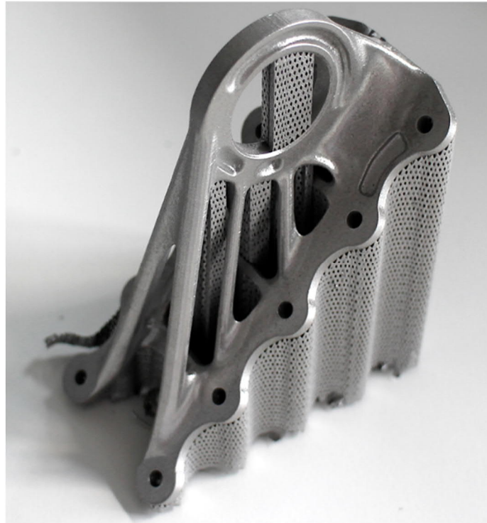
Figure 7. A metal bracket before supports are removed. /11/.
