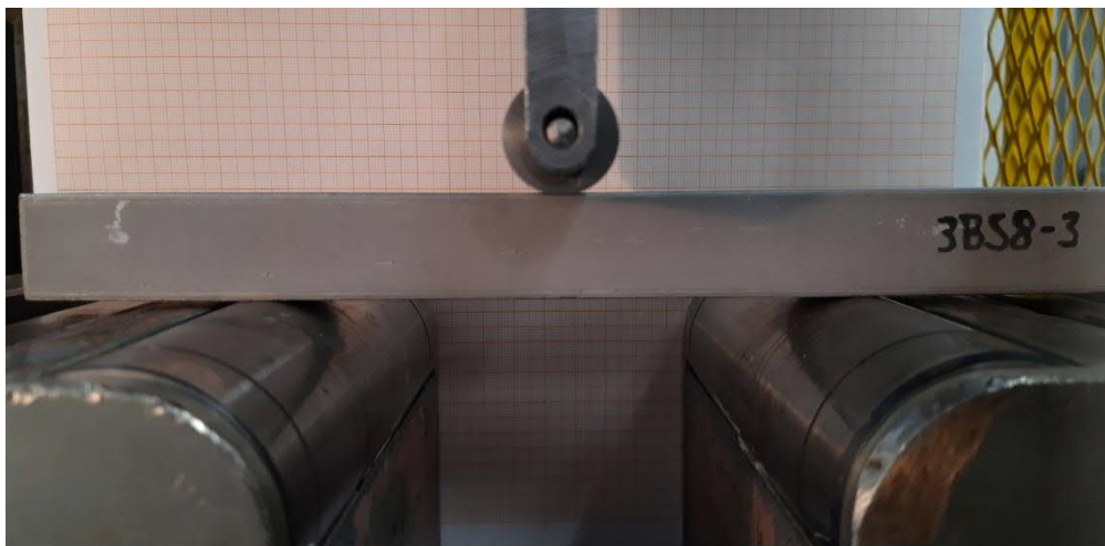
Figure 48. Test sample 3BS8-3 before loading.
