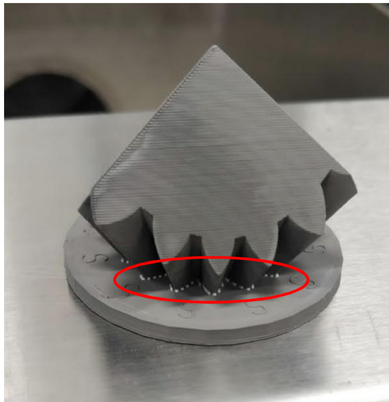
Figure 23. The white ceramic release layer, which makes the part release from the raft easier.
