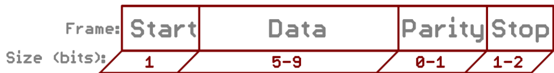
Figure 9. A serial communication packet frame. (Reprinted from [12])
