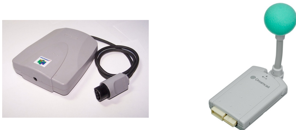
Figure 3. Microphone peripherals for late 1990s game consoles, featuring Voice Recognition Unit (left) for Nintendo 64 and Dreamcast Microphone (right) for Sega Dreamcast (Wikimedia Commons). [35,36]
