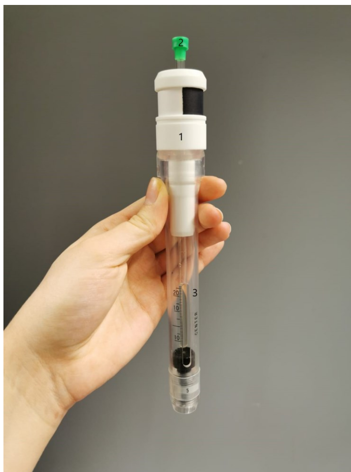
PICTURE 1. The plastic sample holder in the measurement tube. 1. Plastic sample holder 2. Glass tube (sample) 3. Measurement tube
