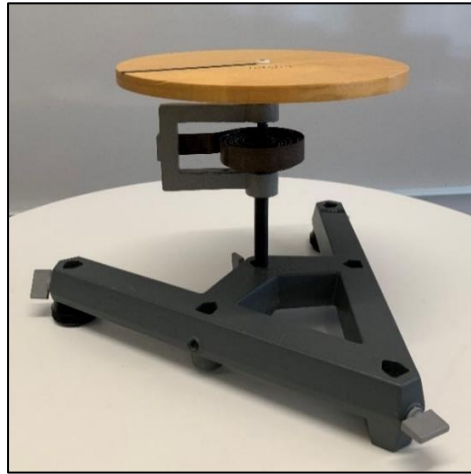
Figure 9: Educational torsional pendulum with wooden disk
