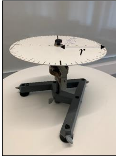
Figure 13: Educational torsional pendulum with metal disk
