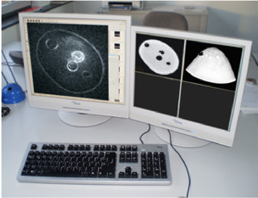
Figure 3. USCT reflection image on the left screen and on right screen a MRT image of the same breast phantom for comparison. [3]
