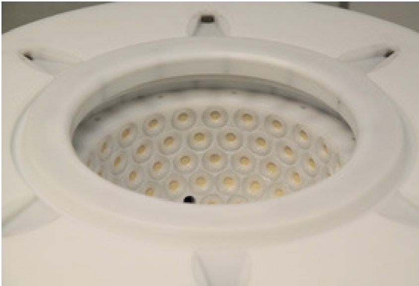
Figure 2. Examination reservoir with mounted transducer arrays filled with water as medium. [3]
