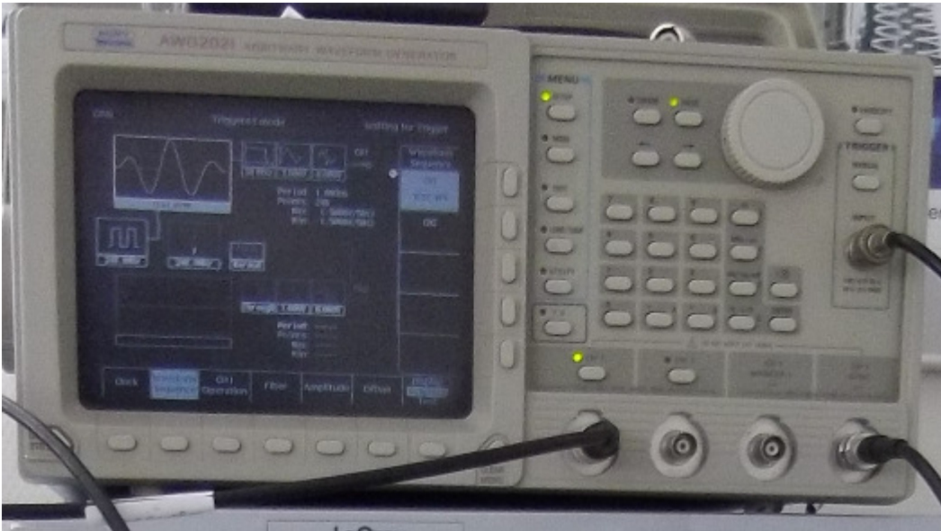
Figure 5. Tektronix AWG2021 arbitrary waveform generator. Information of the parameterized signal on the screen.
