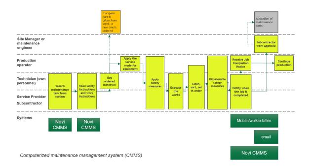
Figure 6. Process flow chart of executing preventive maintenance tasks.
