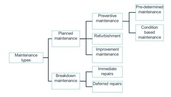
Figure 2. Maintenance types and strategies, adapted from standard PSK 7501
