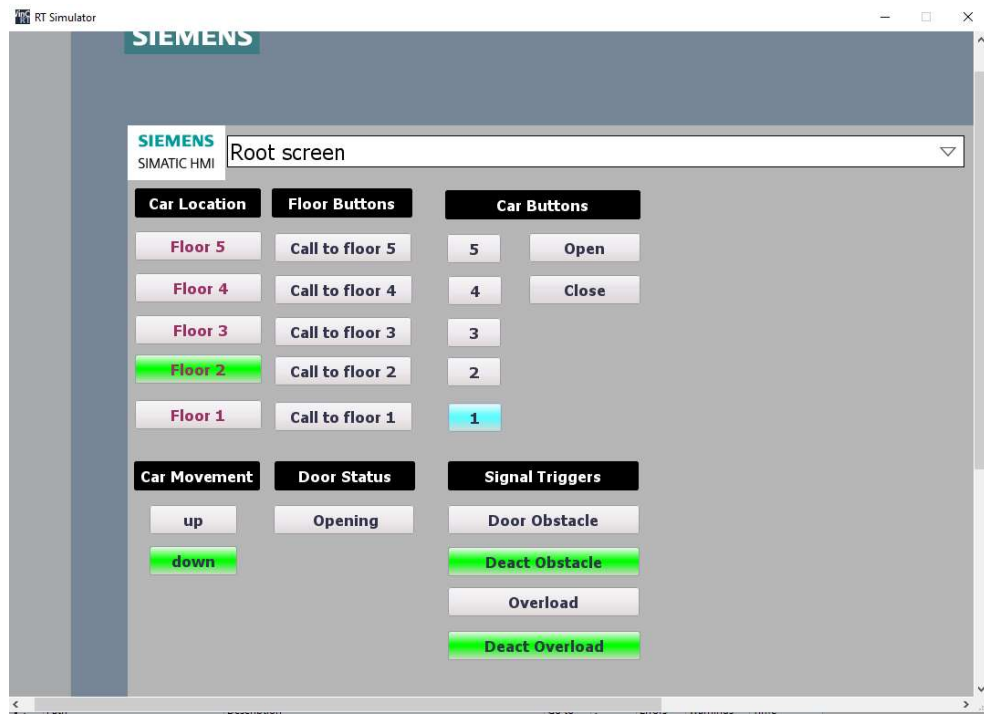
Figure 59. Down movement simulation in HMI screen
