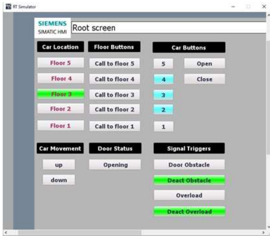
Figure 60. Elevator reached floor 3 and needs to keep moving up
