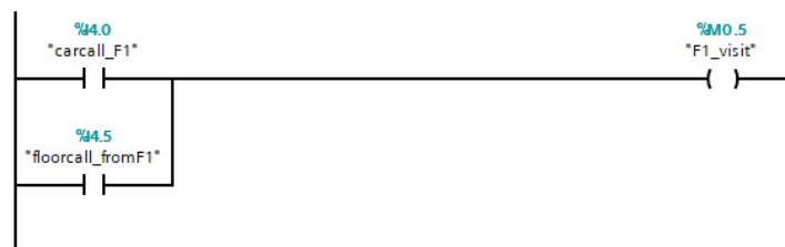
Figure 30. Elevator calls in LAD
