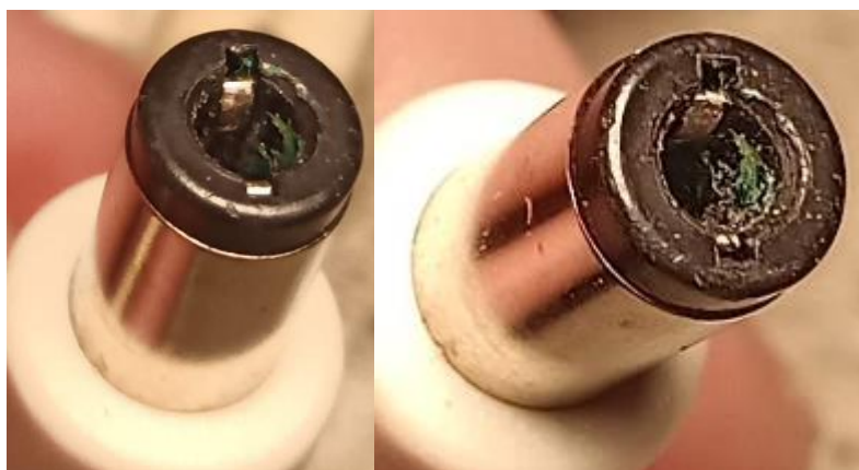
Figure 41. Second plug under test. Green corrosion is apparent.
