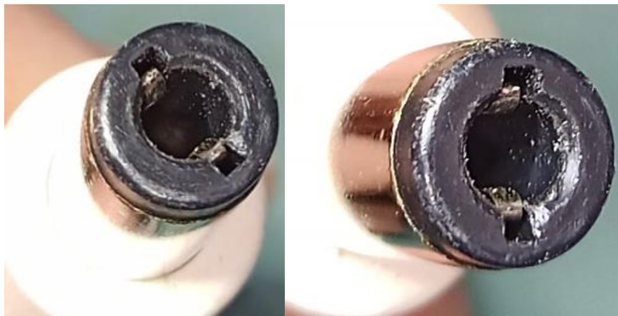
Figure 40. Clean plug that does not contain red phosphorus.
