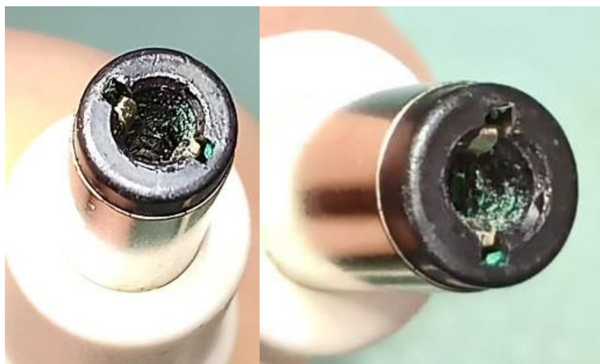
Figure 39. First plug under test. Green corrosion is apparent.
