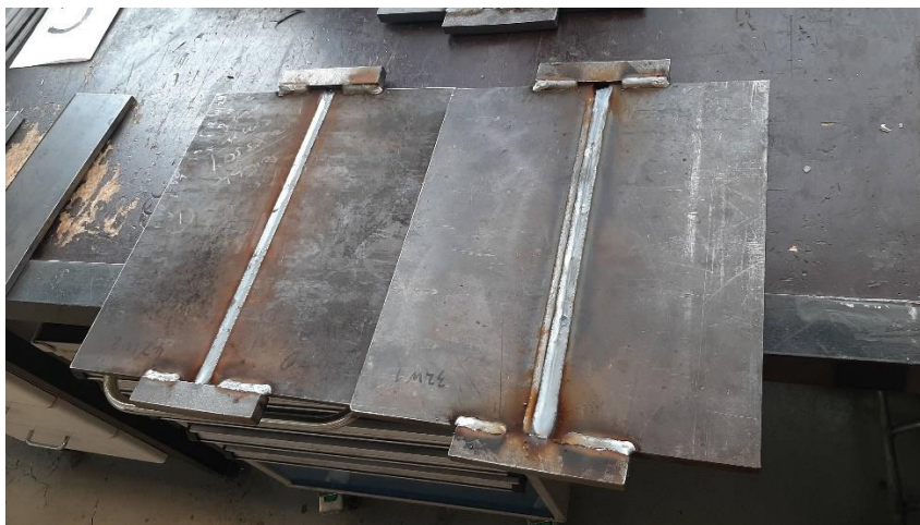
PICTURE 6. Welded E450BR and E350C plates (Paananen 2020.)
