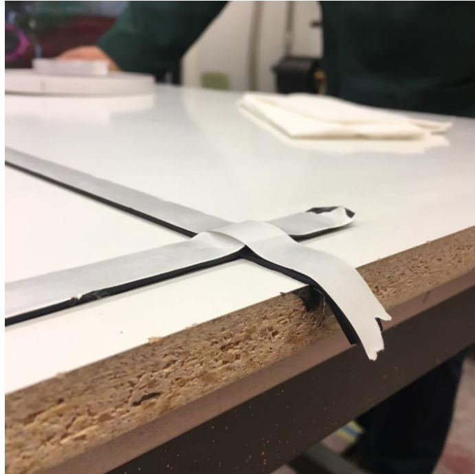
Figure 5 Sealant tape placed on the table
