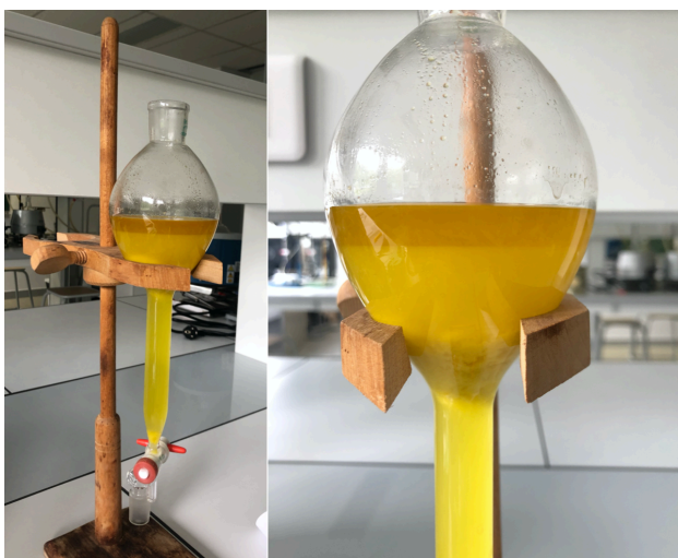
PICTURE 8. Decantation process in separating funnel.
