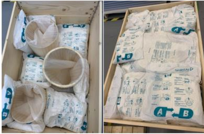
Figure 32. Packing with Instapak. Work on process on the left and ready package on the right.
