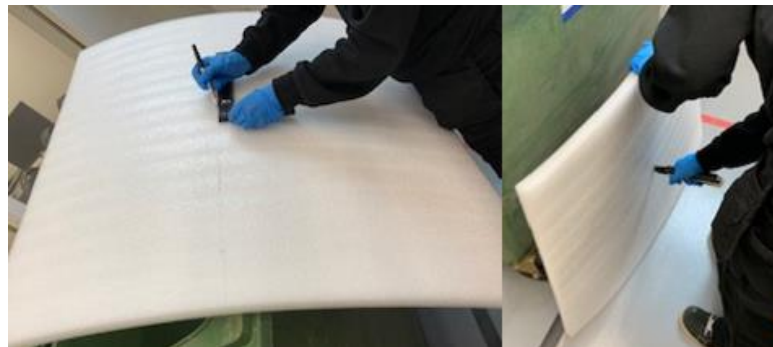
Figure 24. Drawing the measurements of the pallet's bottom and then cutting the piece.
