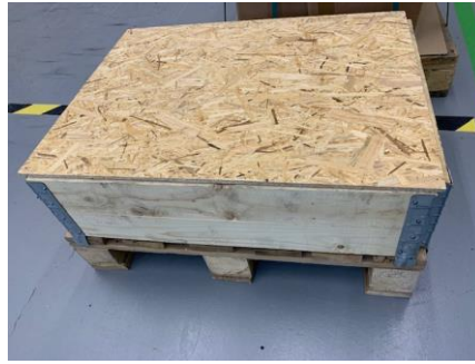
Figure 13. A ready package in Bluefors Oy with a half-pallet, collar and OSB.
