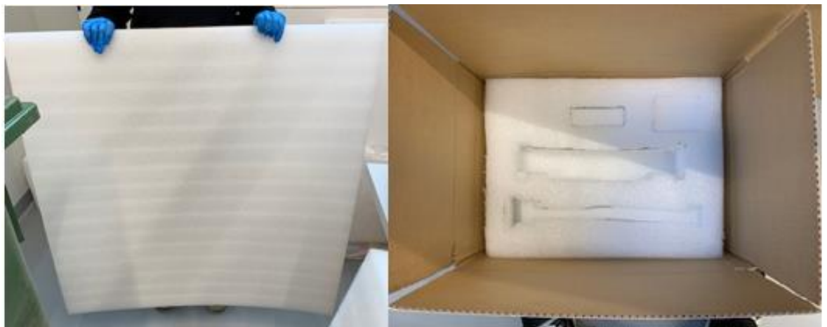
Figure 5. One example of Bluefors' foam blocks (on the left) and a ready hand-carved foam piece in a cardboard box (on the right).
