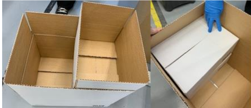
Figure 36. Two pieces of the smallest boxes do not fit properly next to, or on top of each other inside the middle-sized one.
