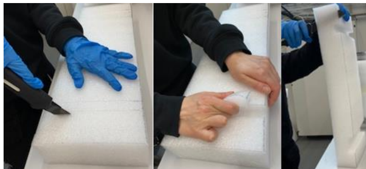
Figure 27. Carving the tracks for the handles of the power supply.
