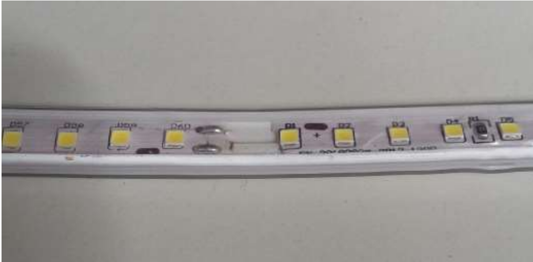
FIGURE 25: Failed LED strip (Elcart) (15.)
