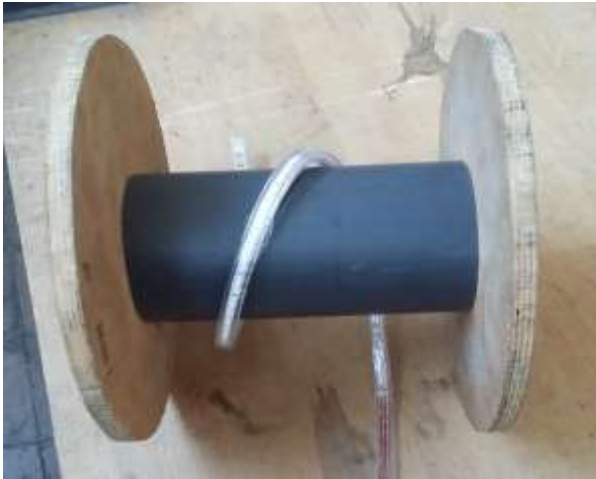
FIGURE 26: Bending tool with 6cm radius (15.)
