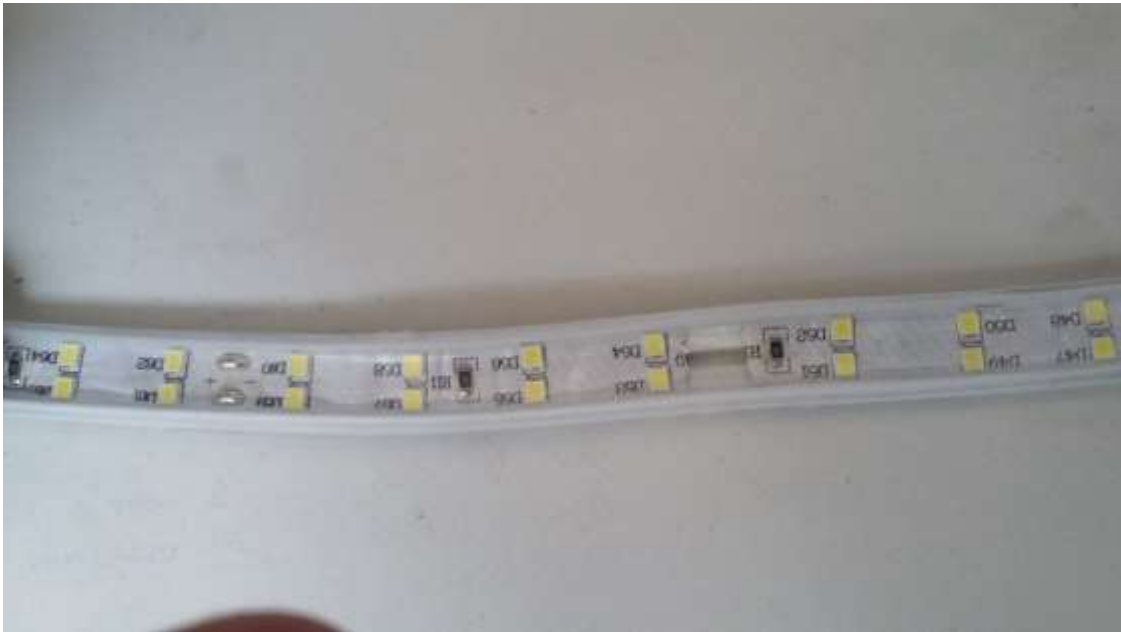
FIGURE 23: Failed LED strip Weco (15.)
