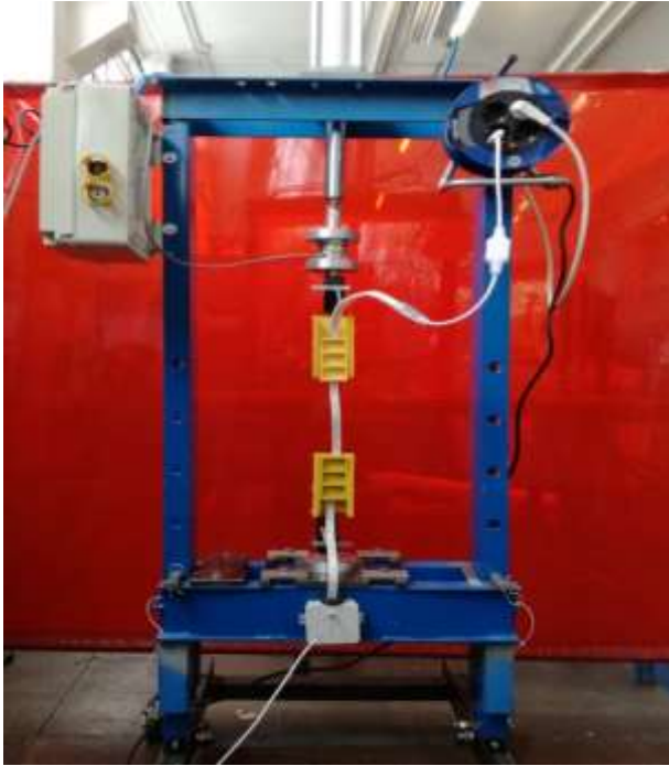
FIGURE 22: Tearing test bench setup (15.)
