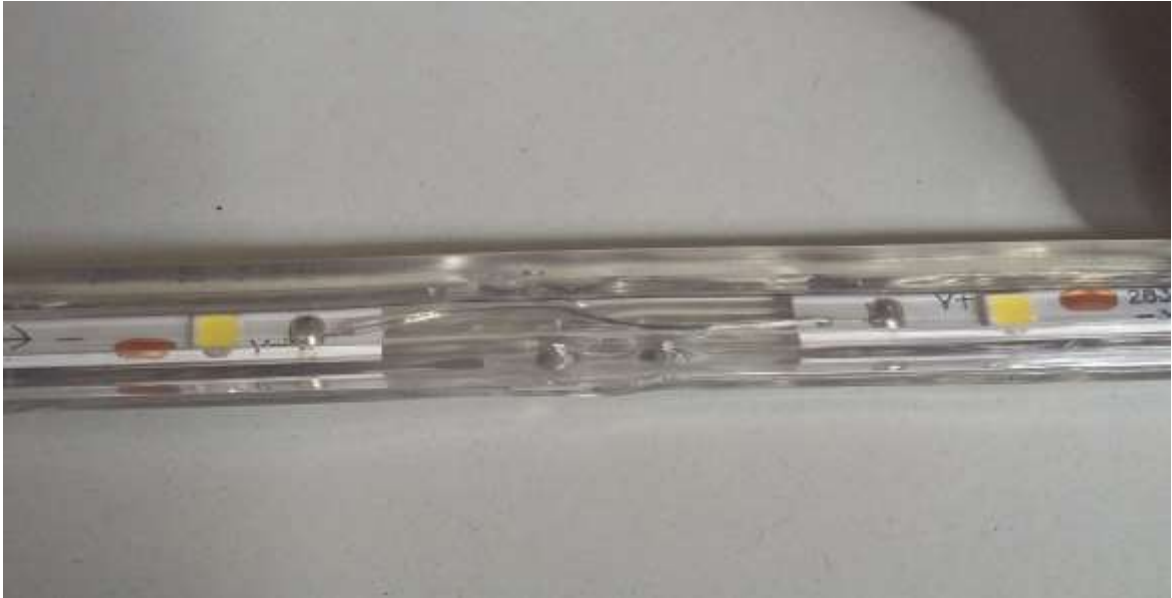
FIGURE 24: Failed LED strip Crosspoint (15.)
