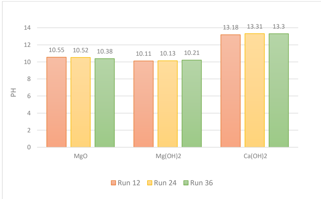
Figure 7. The pH values of different drying media after 12 th , 24 th and 36 th drying runs
